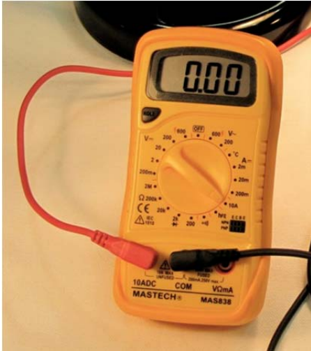
Fig. 1: Multimeter as Ammeter
