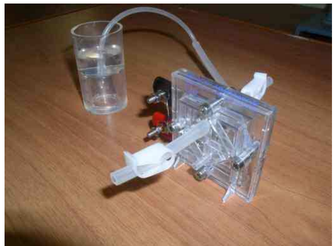
Fig. 7: Reversible proton exchange membrane fuel cell with hydrogen storage (Fuel cell store)
